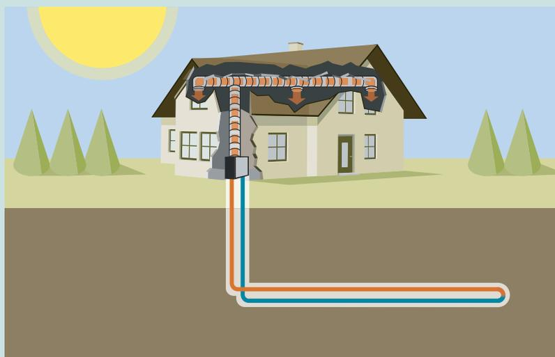
An example of a horizontal loop installation
