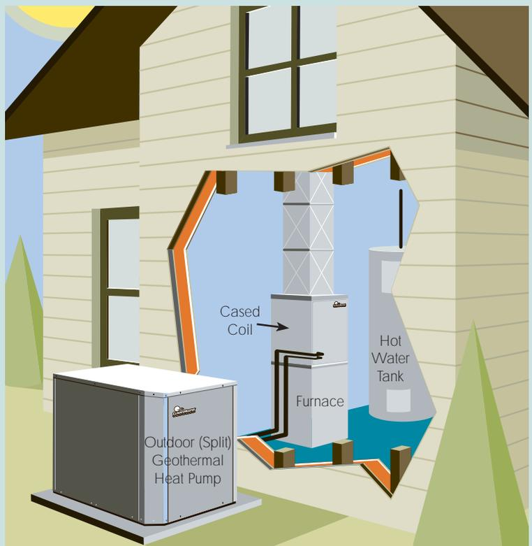
An example of an outdoor dual fuel split unit installation matched with a cased coil
