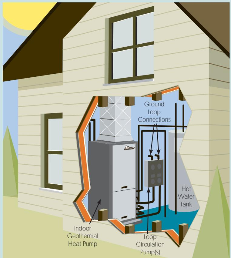
An example of a packaged upflow unit installation
