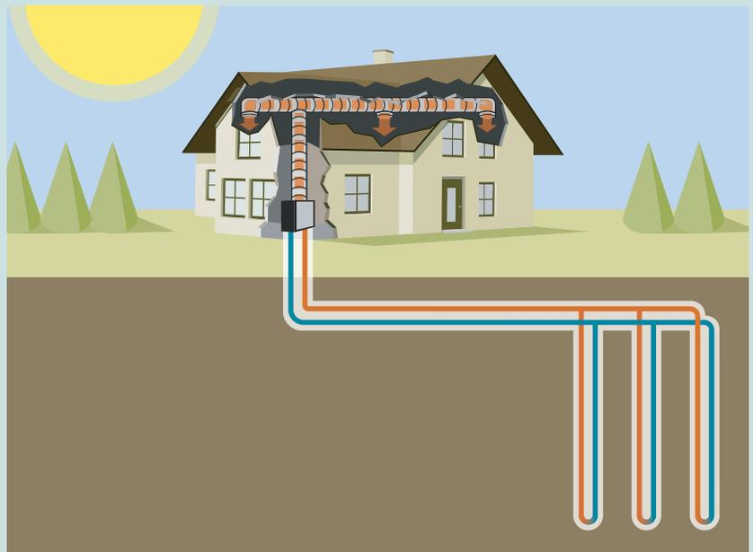
An example of a vertical loop installation
