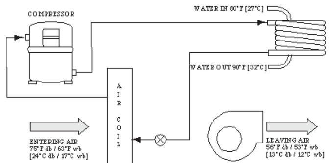
**Figure 5: Typical 100% O/A Reverse Cycle Heat Pump in Heating Mode**
