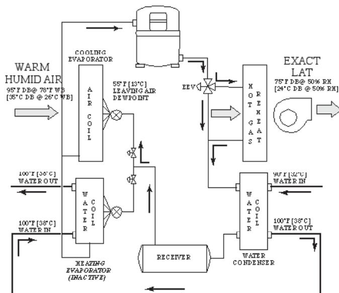
**Figure 8: Schematic with LAT Control:
