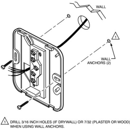
⚠ DRILL 3/16 INCH HOLES (IF DRYWALL) OR 7/32 (PLASTER OR WOOD) WHEN USING WALL ANCHORS.
