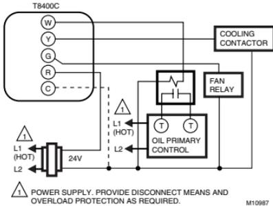
Fig. 6. T8400C heat-cool wiring diagram in oil heating/electric cooling system. Oil primary has its own transformer.
