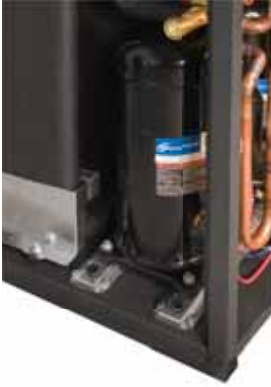
Copeland scroll compressors with dual-isolation mounting for quiet operation
