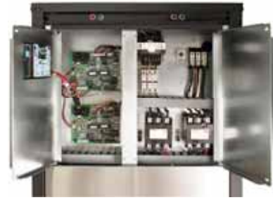
Advanced digital controls with Remote Service Sentinel and compressor "run" and "fault" LED. Optional Enhanced controls (DXM) & DDC Controllers
